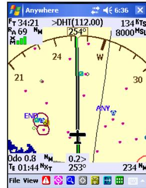
14. Airway segments with multiple victor airway names do not over-write one another as in the past. In the case of overlapping victor airways on the same segment, the multiple airway numbers are shown hyphenated, such as "V74-516" shown at right. The MEA is still shown underneath.
