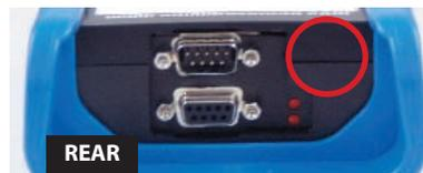
On Power-up (battery or external) both lights are ON for 5 seconds.
